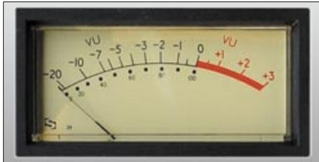
The VU meters have a leave of 4 dB as a standard. In standard nominal level +6 dBu there is 100% = 0dB indication of the VU meter at level +2 dBu. But there are also other settings possible.
